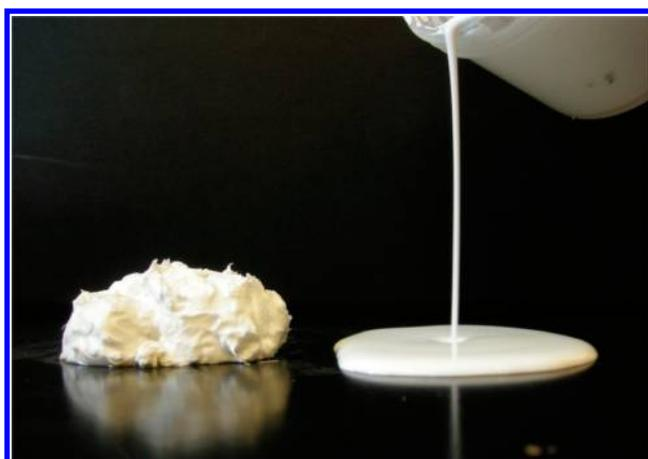
Figure 8. Silica particle ( $1\ \mu\text{m}$ ) suspension bridge flocculated by PEO MW  $4 \times 10^6$  g/mol before and after the mixing in SpeedMixer for 6 min at 3300 rpm.
