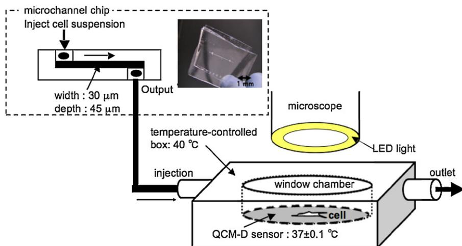
Fig. 1. Schematic illustration of cell-analytical system.
