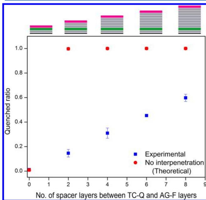
**Figure 3.** Quenched ratio of DNA multilayer films assembled by depositing alternating 0, 2, 4, 6, and 8 nonfluorescent spacer polyA<sub>15</sub>G<sub>15</sub> and polyT<sub>15</sub>C<sub>15</sub> layers between TC-Q and AG-F layers on polyT<sub>30</sub>/polyA<sub>15</sub>G<sub>15</sub> layers.
