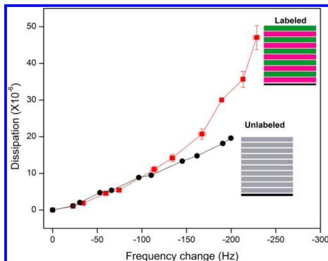
**Figure 1.** Comparison between the growth of a 5-bilayer labeled (polyT<sub>30</sub>/(AG-F/TC-Q)<sub>5</sub>) and unlabeled (polyT<sub>30</sub>/(polyA<sub>15</sub>G<sub>15</sub>/polyT<sub>15</sub>C<sub>15</sub>)<sub>5</sub>) film, as monitored using QCM. The polyT<sub>30</sub>, TC-Q, and AG-F layers are represented by black, green, and pink lines, respectively.
