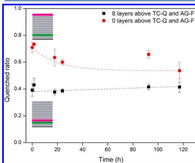
**Figure 6.** Quenched ratio of a 5-bilayer film (with no layers above the TC-Q and AG-F layers or with eight nonfluorescent layers above the TC-Q and AG-F layers) as a function of time. The dotted lines are to guide the eye.
