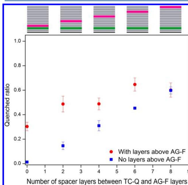
**Figure 5.** Quenched ratio of a 5-bilayer film with increasing number of layers between the TC-Q and AG-F layers (represented as red dots; scheme on top of plot). The blue squares represent the quenched ratio of the film with the same number of layers between the TC-Q and AG-F layers but without additional layers above the AG-F layer.
