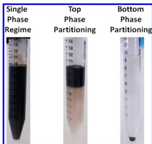
**Figure 2.** Possibilities of the partitioning behavior of 100 nm silica particles in an Eumulgin ES-based AMTPS: (left) in a single-phase state, the particles are homogeneously distributed in the solution; (middle) the particles partition into the micelle-rich top phase; and (right) the particles partition into the micelle-poor bottom phase and sediment on the bottom.
