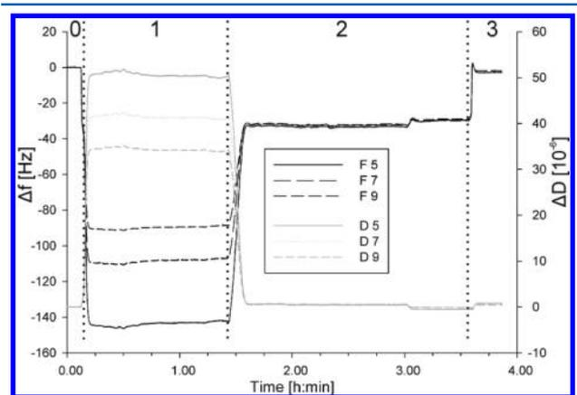
**Figure 3.** QCM-D signal obtained during the rinsing of a silica chip with sodium citrate and Eumulgin ES at pH 3 and 20 °C. The silica chip is rinsed with (0) sodium citrate, (1) 10% Eumulgin ES in sodium citrate, (2) sodium citrate, and (3) Milli-Q water. The signal shift to  $-35$  Hz is generated by a Eumulgin ES monolayer that is adsorbed to the silica surface. When the chip is rinsed with Milli-Q water, the Eumulgin ES layer is removed completely.
