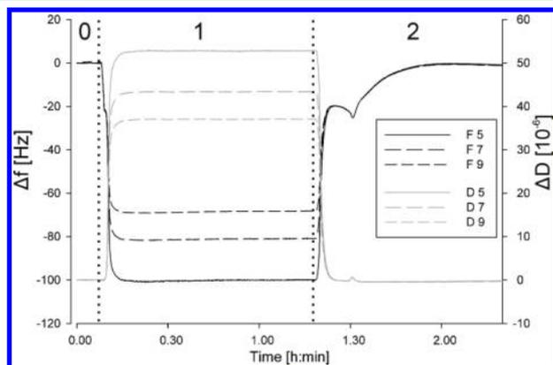
**Figure 7.** QCM-D signal obtained during rinsing a silica chip with sodium citrate, 6 M urea, and Eumulgin ES at pH 3 and 20 °C. The silica chip is rinsed with (0) sodium citrate, 6 M urea, pH 3; (1) 10% Eumulgin ES in sodium citrate, 6 M urea, pH 3; and (2) sodium citrate, 6 M urea, pH 3. Eumulgin ES is completely removed from the chip surface after rinsing with the buffered urea solution.
