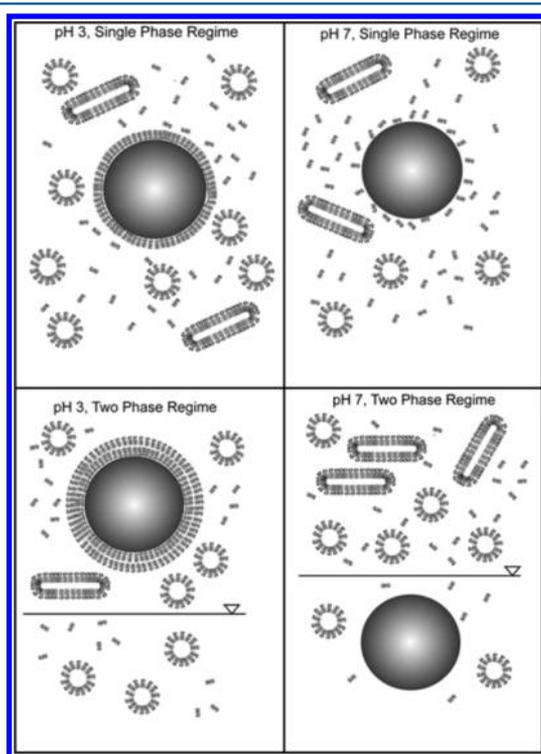
**Figure 12.** Mechanism of the partitioning of an insoluble particle in AMTPS. If the phase-forming surfactant adsorbs to the particle, then it is drawn to the micelle-rich phase. If the surfactant does not adsorb to the particle surface, then the particle is expelled from the micelle-rich phase.
