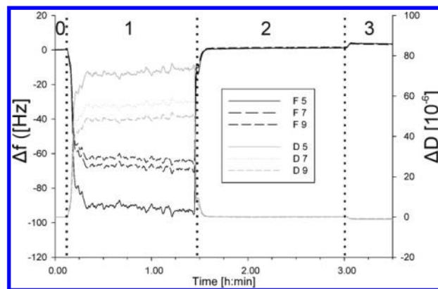
**Figure 4.** QCM-D signal obtained during the rinsing of a silica chip with sodium phosphate and Eumulgin ES at pH 7 and 20 °C. The silica chip is rinsed with (0) sodium phosphate, (1) 10% Eumulgin ES in sodium phosphate, (2) sodium phosphate, and (3) Milli-Q water. Eumulgin ES is completely removed from the chip surface after it is rinsed with sodium phosphate.
