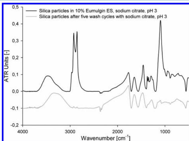
**Figure 10.** ATR-FTIR spectra of MagPrep silica particles incubated with Eumulgin ES at pH 3. The peaks at 2800–2950 cm<sup>-1</sup> are generated from CH<sub>2</sub> and CH<sub>3</sub> stretching caused by surfactant hydrocarbon chains at the particle surface. Peaks can still be observed on the particle surface after five wash cycles at pH 3.
