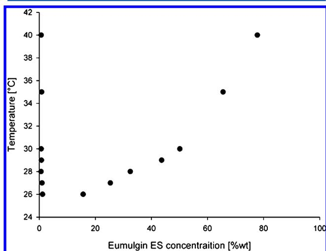
**Figure 1.** Phase diagram of a 20 mM sodium citrate Eumulgin ES AMTPS. The points of transition from a single-phase to a two-phase state are shown. The phase separation depends on the surfactant concentration and the temperature.
