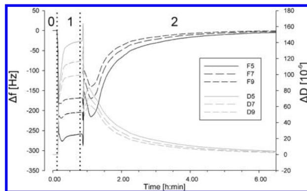
**Figure 8.** QCM-D signal obtained during rinsing a silica chip with sodium citrate, 6 M urea, and Eumulgin ES at pH 3 and 35 °C. The silica chip is rinsed with (0) sodium citrate, 6 M urea, pH 3; (1) 10% Eumulgin ES in sodium citrate, 6 M urea, pH 3; and (2) sodium citrate, 6 M urea, pH 3. The obtained signals converge to zero; no surfactant is adsorbed permanently to the silica surface.
