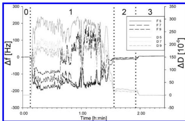
**Figure 6.** QCM-D signal obtained from rinsing a silica chip with sodium phosphate and Eumulgin ES at pH 7 and 30 °C. The silica chip is rinsed with (0) sodium phosphate, (1) 10% Eumulgin ES in sodium phosphate, (2) sodium phosphate, and (3) Milli-Q water. Eumulgin ES is completely removed from the chip surface after it is rinsed with sodium phosphate at 30 °C.
