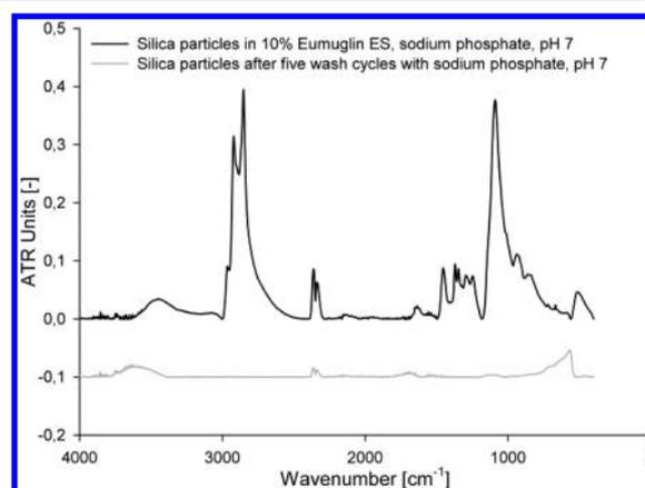
**Figure 11.** ATR-FTIR spectra of MagPrep silica particles incubated with Eumulgin ES at pH 7. The peaks at 2800–2950 cm<sup>-1</sup> are generated from CH<sub>2</sub> and CH<sub>3</sub> stretching caused by surfactant hydrocarbon chains at the particle surface. These peaks cannot be observed on the particle surface after five wash cycles at pH 7.
