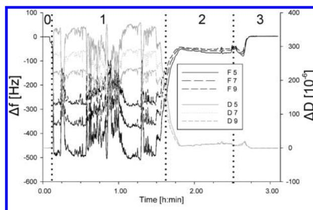
**Figure 5.** QCM-D signal obtained during rinsing a silica chip with sodium citrate and Eumulgin ES at pH 3 and 30 °C. The silica chip is rinsed with (0) sodium citrate, (1) 10% Eumulgin ES in sodium citrate, (2) sodium citrate, and (3) Milli-Q water. A signal shift of  $-55$  Hz emerges when the surface is flushed with sodium citrate. The signal comes from a stable surfactant double layer formed on the silica surface at pH 3 and 30 °C.
