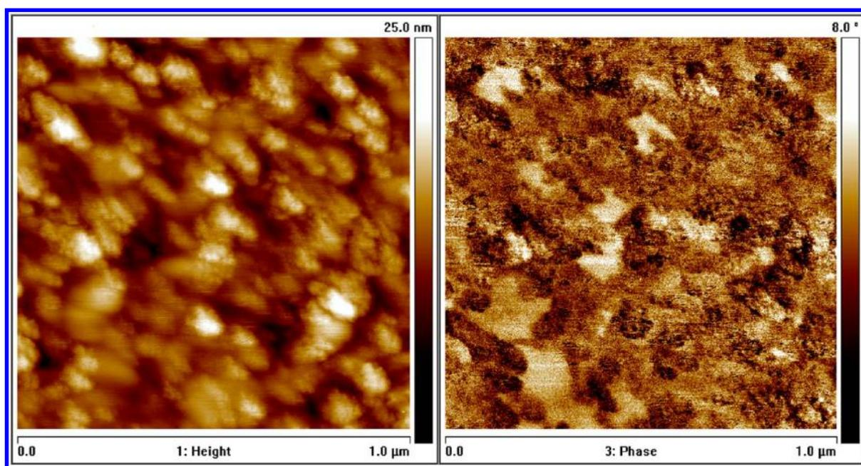
**Figure 5.** AFM topographic images of the brush grown from an initial SAM containing 5% thiol initiator; image contrast in terms of height and phase.
