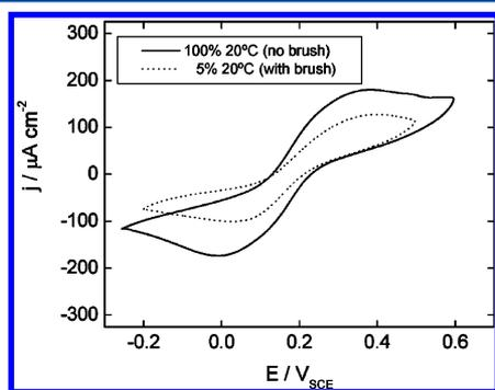
**Figure 4.** Cyclic voltammograms for an electrode modified with an initial SAM containing 100% thiol initiator ( $-$ ) and for a second electrode modified with an initial SAM containing 5% thiol initiator from which the PNIPAM brush was grown ( $\cdots$ ). Voltammograms were recorded at a sweeping rate of  $50 \text{ mV s}^{-1}$  and at  $20$   $^{\circ}\text{C}$ .
