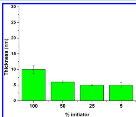
**Figure 12.** Ellipsometric thicknesses of PNIPAM brushes grown from thiol monolayers with different percentages of initiator as measured in the dry state.
