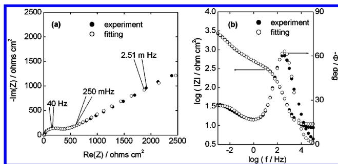
**Figure 7.** Impedance spectra for an electrode modified with an initial SAM containing 100% thiol initiator without subsequent brush growth. Measured and fitted data represented as Nyquist diagrams (a) and Bode plots (b). Experimental data (●) and fit results (○) according to the equivalent circuit (Figure 11a) and the reaction impedance  $Z_f$  from eq 7.
