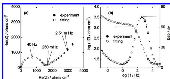
**Figure 8.** Impedance spectra for an electrode modified with an initial SAM containing 5% thiol initiator from which the PNIPAM brush was grown. Measured and fitted data represented as Nyquist diagrams (a) and Bode plots (b). Experimental data (●) and fit results (○) according to the equivalent circuit (Figure 11a) and the reaction impedance  $Z_f$  from eq 7.
