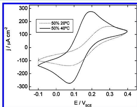
**Figure 3.** Cyclic voltammograms for a single electrode modified with a PNIPAM brush grown from an initial SAM containing 50% thiol initiator. Voltammograms were recorded at a sweeping rate of  $50 \text{ mV s}^{-1}$  and at two electrolyte temperatures  $20$  ( $\cdots$ ) and  $40$   $^{\circ}\text{C}$  ( $-$ ).
