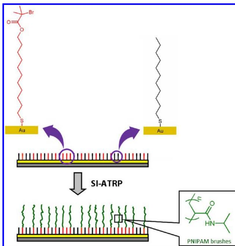
**Figure 1.** Schematic representation of a Au substrate modified with an initial SAM containing a mixture of initiator/inhibitor thiols (upper sketch) and the resulting surface after growth of a PNIPAM brush via ATRP (lower sketch).
