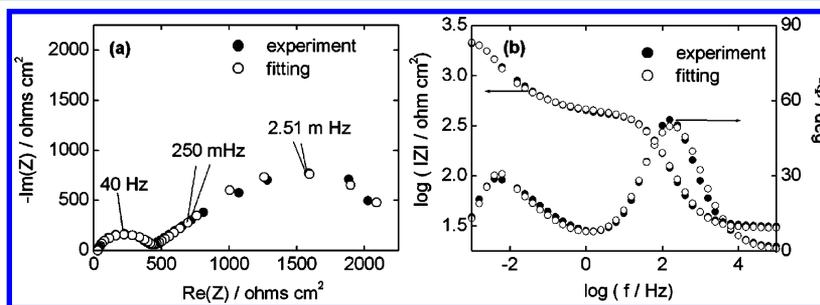
**Figure 9.** Impedance spectra recorded at 20 °C for an electrode modified with an initial SAM containing 50% thiol initiator from which the PNIPAM brush was grown. Experimental data (●) and fit results (○) according to the equivalent circuit (b) and the reaction impedance  $Z_f$  from eq 6.
