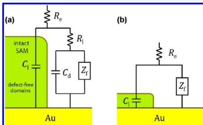
**Figure 11.** Schematic representation of an electrode modified with a SAM from which the PNIPAM brushes were grown. The SAM contains defects exposing the bare Au surface. The corresponding equivalent circuit is presented in its general form (a) and in a simplified form (b).
