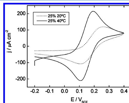
**Figure 2.** Cyclic voltammograms for a single electrode modified with a PNIPAM brush grown from an initial SAM containing 25% thiol initiator. Voltammograms were recorded at a sweeping rate of 50 mV s<sup>-1</sup> and at two electrolyte temperatures 20 (···) and 40 °C (—).
