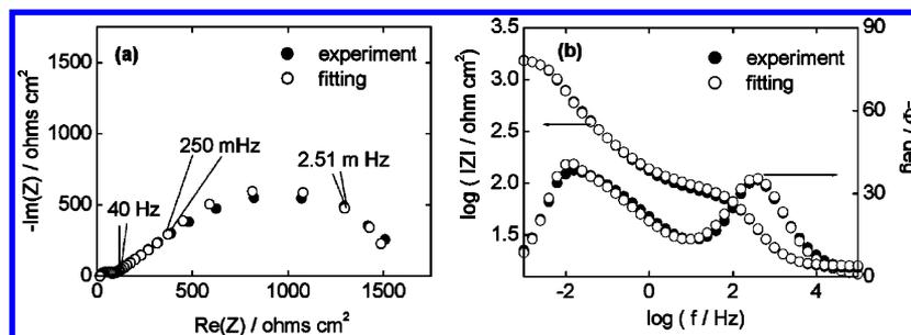
**Figure 10.** Impedance spectra recorded at 40 °C for an electrode modified with an initial SAM containing 50% thiol initiator from which the PNIPAM brush was grown. Experimental data (●) and fit results (○) according to the equivalent circuit (Figure 9b) and the reaction impedance  $Z_f$  from eq 6.
