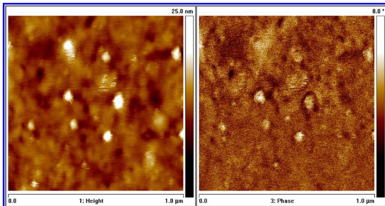
**Figure 6.** AFM topographic images of the brush grown from an initial SAM containing 100% thiol initiator; image contrast in terms of height and phase.
