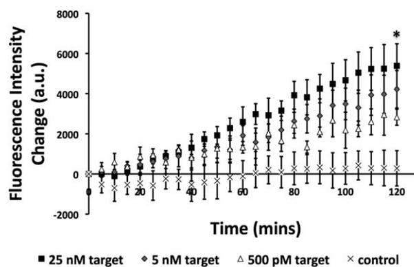
**Fig. 5** Detection responses from 12 microfluidic channels upon introduction of target DNA solutions containing different concentrations (25 nM, 5 nM, 500 pM, and 0 M target). Data are presented as mean  $\pm$  standard deviation.  $N = 3$  (3 microfluidic channels). CCD exposure time: 10 s. Statistical analysis was performed using one-way ANOVA with *tukey post hoc* test, Matlab.  $N = 3$  (3 channels). (\*) Significant difference was found between any two groups.
