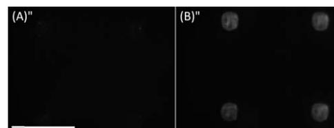
**Fig. 3** Fluorescence microarray images showing the signals from four identical *Bacillus anthracis* probe spots on the channel floor (A) before and (B) after exposure to a 2.5  $\mu\text{M}$  target solution that was introduced into the channel at a velocity of 0.5  $\mu\text{l min}^{-1}$  for 30 min. Scale bar: 250  $\mu\text{m}$ . CCD exposure time: 10 s.
