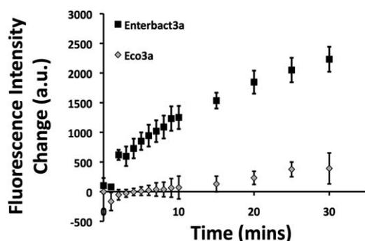
**Fig. 6** Real-time fluorescence responses during a continuous target flow for a multiplex sensor. The 500 nM synthetic Enterbact3a target DNA solution was delivered to the device at a speed of  $0.5 \mu\text{L min}^{-1}$  for 30 min. Data are presented as mean  $\pm$  standard deviation.  $N = 3$  (3 microfluidic channels). CCD exposure time: 10 s.
