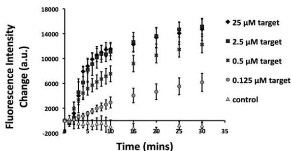
**Fig. 4** Real-time fluorescence intensity changes as a function of different target concentrations. Data are presented as mean  $\pm$  standard deviation.  $N = 3$  (3 microfluidic channels). CCD exposure time: 10 s.
