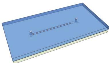
**Fig. 2** Schematic of the simple microfluidic device employed in this study. The PDMS microchannel is covalently bonded to an Ag nanoparticle surface carrying an array of DNA hairpin probe spots (represented by circles). Spot size, number of spots, and channel dimensions are not drawn to scale.
