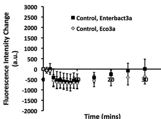
**Fig. 7** Fluorescence intensity changes from 6 microfluidic channels upon introduction of buffer only into the device at a velocity of  $0.5 \mu\text{L min}^{-1}$  for 30 min. Substrate surfaces were arrayed with Enterbact3a and Eco3a probes. Data are presented as mean  $\pm$  standard deviation.  $N = 3$  (3 microfluidic channels).
