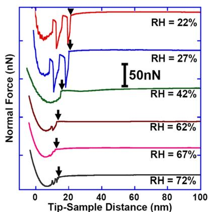
FIG. 3. (Color online) Force-distance curves with different RH values without lateral modulation at a tip-speed of 8 nm/s. The oscillatory force decreases drastically at humidities above RH 42%. The arrows point to the distance where two water structures meet between the two surfaces.
