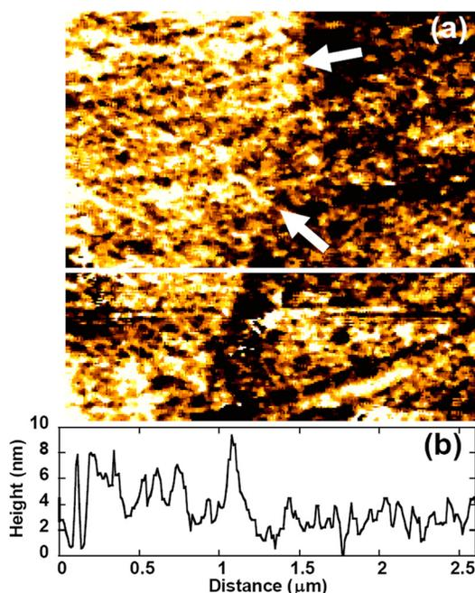
FIG. 4. (Color online) (a) Non-contact AFM image of water structures on the silicon surface at RH = 47% (scan area:  $2.5 \mu\text{m} \times 2.5 \mu\text{m}$ ). (b) A sectional profile along the white line above shows that water clusters are up to 8–10 nm high.
