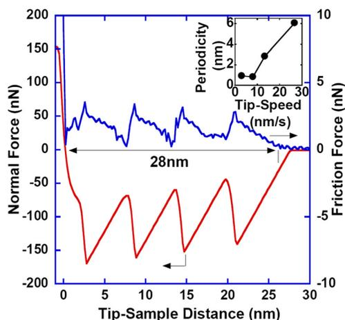
FIG. 2. (Color online) Measurement taken at a lower time-scale of 30 s at a tip-speed of 27 nm/s at RH 33%. (inset) The periodicity in relation to the varying tip-speeds.
