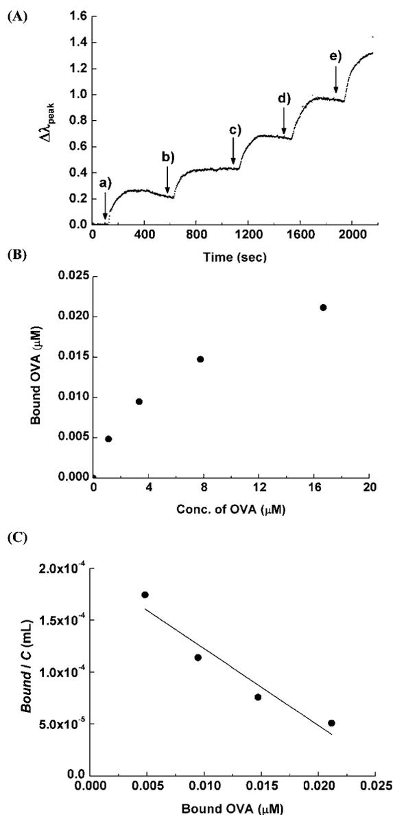
**Fig. 4** (A) Cumulative change in  $\Delta\lambda_{\text{peak}}$  values after the consecutive OVA injections: (a) 0.05, (b) 0.1, (c) 0.2, (d) 0.4 and (e) 0.5  $\text{mg mL}^{-1}$ . (B) Binding isotherm of OVA of the Con A-immobilized silicon nitride chip based on the change in optical thickness calculated from the  $\Delta\lambda_{\text{peak}}$  values.<sup>10</sup> (C) Scatchard plot from the binding data of OVA.
