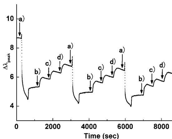
**Fig. 6** Monitoring of the regeneration process by the concentration-dependent change in  $\Delta\lambda_{\text{peak}}$  against the injections of (a) 10 mM glycine-HCl (pH 1.5), (b) 0.05 mg mL<sup>-1</sup>, (c) 0.1 mg mL<sup>-1</sup>, and (d) 0.2 mg mL<sup>-1</sup> of OVA solutions.
