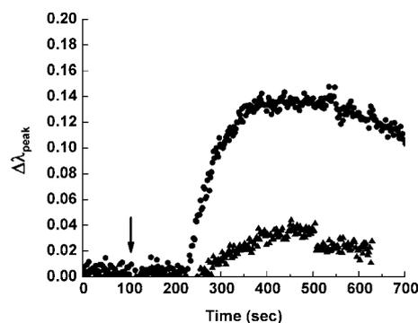
**Fig. 3** Real time monitoring of  $\Delta\lambda_{\text{peak}}$  values after the injection (100  $\mu\text{L}$ ) of OVA (0.1 mg mL<sup>-1</sup>) (circles) and BSA (0.1 mg mL<sup>-1</sup>) (triangles). Running buffer: 10 mM HEPES (pH 7.4) buffer containing 150 mM NaCl, 1 mM CaCl<sub>2</sub> and 1 mM MnCl<sub>2</sub>. Flow rate: 20  $\mu\text{L min}^{-1}$ .
