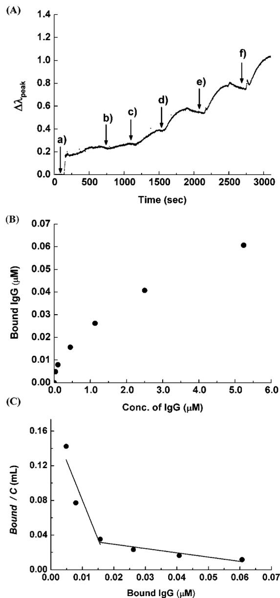
**Fig. 5** (A) Cumulative change in  $\Delta\lambda_{\text{peak}}$  values after the consecutive OVA injections: (a) 0.005, (b) 0.01, (c) 0.05, (d) 0.1, (e) 0.2 and (f) 0.4  $\text{mg mL}^{-1}$ . (B) Binding isotherm of rabbit IgG on the Con A-immobilized silicon nitride chip based on the change in optical thickness calculated from the  $\Delta\lambda_{\text{peak}}$  values.<sup>10</sup> (C) Scatchard plot from the binding data of rabbit IgG.
