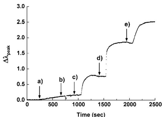
**Fig. 2** *In situ* monitoring of the surface modification by the change in  $\Delta\lambda_{\text{peak}}$  values after injections of (a) NHS-PEG<sub>4</sub>-Biotin, (b) changing buffer from 100 mM sodium borate buffer (pH 8.5) to 10 mM PB (pH 7.4), (c) BSA blocking, (d) avidin binding, and (e) immobilization of biotinylated Con A.
