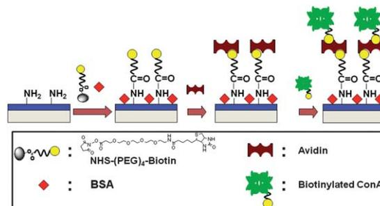
**Fig. 1** Schematic illustration of biotinylated Con A immobilization via avidin–biotin interaction on a silicon nitride chip.
