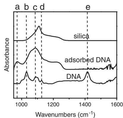
**Fig. 3.** FTIR spectroscopy of silica (top), DNA adsorbed on silica (middle) and dissolved chromosomal DNA (bottom), all in the presence of 1 mM  $\text{Ca}^{2+}$ . The observed vibrational modes are 971 (a: DNA backbone absorption peak), 1030 (b: DNA backbone absorption peak), 1087 (c: symmetrical  $\text{PO}_2^-$  stretching mode), 1126 (d: asymmetric  $\text{PO}_2^-$  stretching mode), and 1416 (e: base pair absorption peak).
