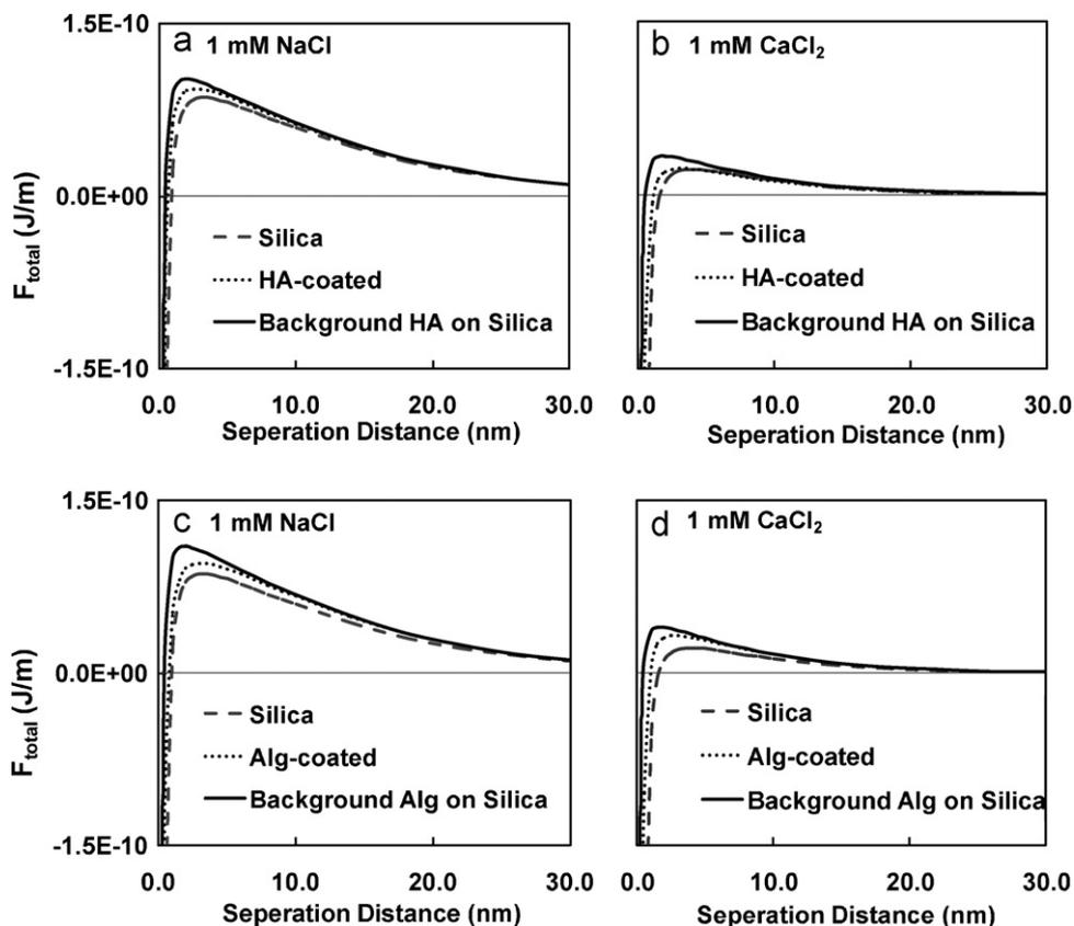
**Fig. 3.** DLVO interaction forces between EPS and bare silica surface in the presence and absence of background NOM and between EPS and NOM-coated surface in the absence of background NOM in 1 mM NaCl and 1 mM CaCl<sub>2</sub> solutions. The EPS size, zeta potentials of EPS and collectors utilized to calculate DLVO interaction forces are listed in Table S4.
