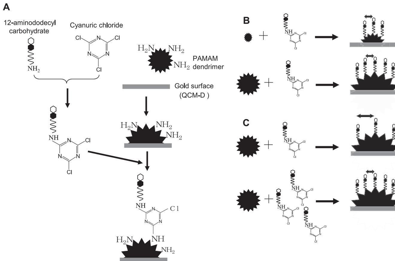
**Fig. 1.** (A) Schematic depicting the immobilization of a carbohydrate molecule on a PAMAM-adsorbed sensor surface for QCM-D studies. The cluster sizes and densities of carbohydrates immobilized on the sensor surface can be controlled by adjusting (B) the size of the PAMAM dendrimers or (C) the density of carbohydrates immobilized on the dendrimers.
