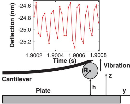
FIG. 1. (Color online) Schematic of a cantilever defining symbols used in the text. The inset shows a 0.6 ms sample of deflection fluctuations at a probe-plate separation of  $\sim 1 \mu\text{m}$  in an experiment with  $k = 0.067 \text{ N/m}$  and  $R = 10.3 \mu\text{m}$ .
