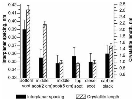
Fig. 2 Average interplanar spacing and crystallite length for different soot particles
