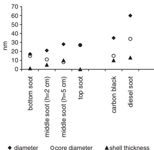
**Fig. 4** Average particle sizes, core diameters, and shell thicknesses of different flame soot particles, carbon black and diesel soot
