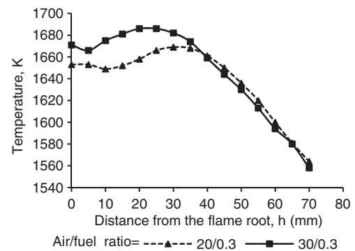
Fig. 3 Measured temperature profile of a flame along the central axis for two different air/fuel ratios. All the subsequent analyses are for the particles collected at air/fuel ratio = 30/0.3
