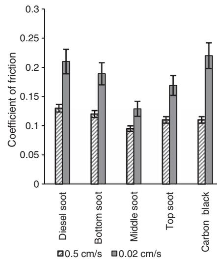
**Fig. 8** Coefficients of friction from dry tribology test involving different soot samples for the linear speeds of 0.5 and 0.02 cm/s
