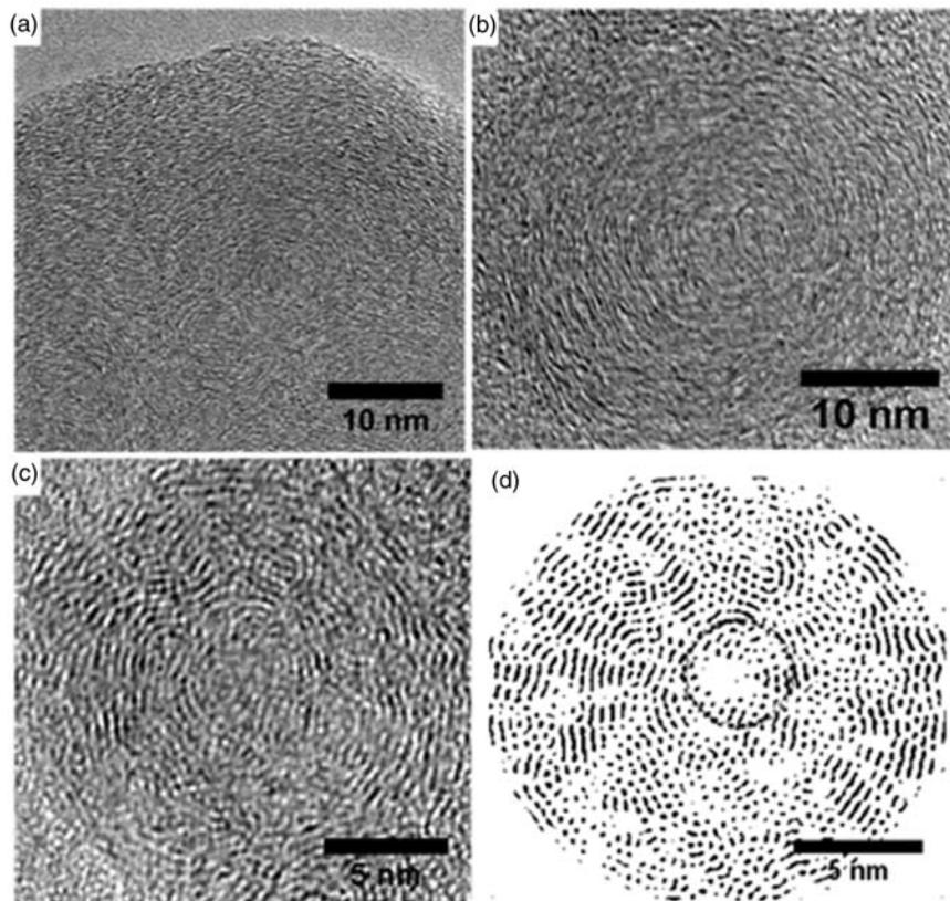
**Fig. 1** Structures of (a) diesel soot, (b) carbon black, and (c) mid-flame soot; (d) processed HRTEM image of mid-flame soot particle showing inner core and outer shell
