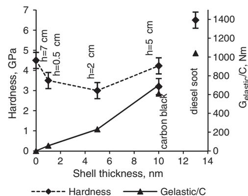
**Fig. 5** Hardness and elastic energy as the function of ordered graphitic shell thickness of different soot particles, where  $C$  is a geometric constant and the estimate of elastic energy is as per the formulation of Hurt *et al.* [23]
