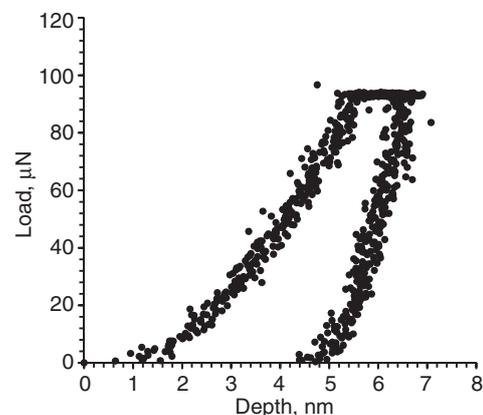
Fig. 9 Typical load–depth curve of flame soot
