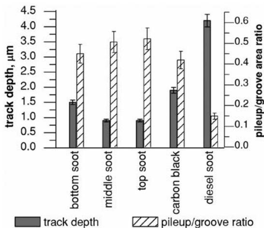
**Fig. 7** Pile-up area/groove area,  $\rho$  and groove depth values measured for wear tracks (speed = 0.5 cm/s)
