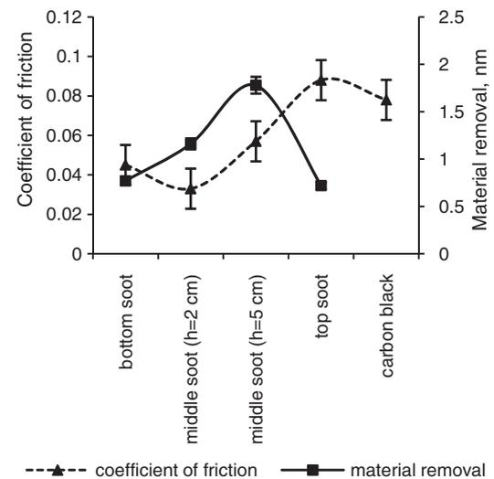
Fig. 6 Coefficients of friction and material removal at normal load of 200 nN, for different types of soot measured by LFM
