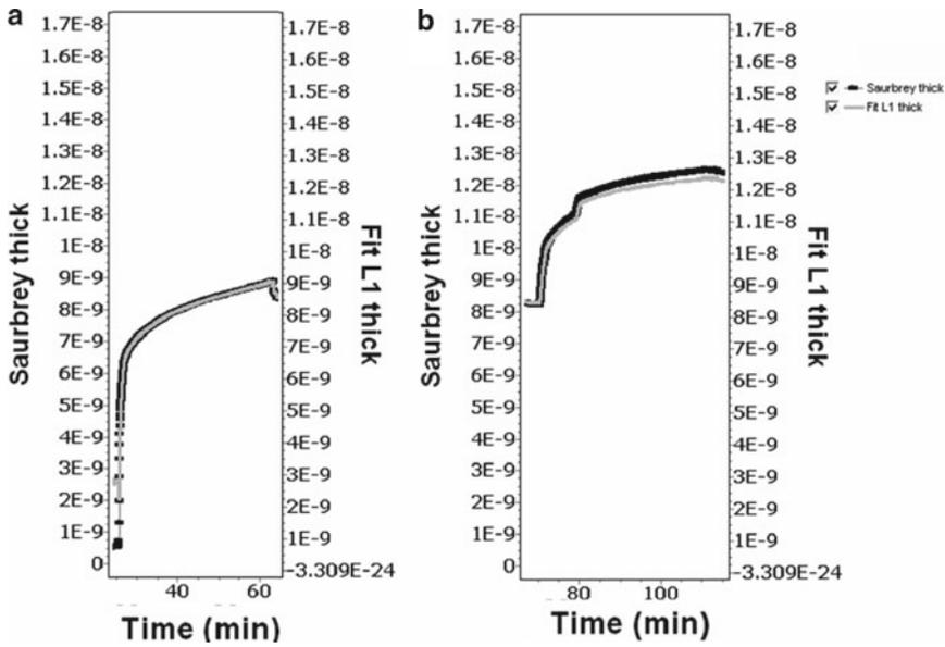
Fig. 2. Fit analysis for the adsorption of C3 onto VCP adsorbed onto PS. The values of Saurbrey thickness (Y1-axis) and Fit L1 thickness (Y2-axis) obtained after Fit analysis done using the QTools software coincide with each other indicating that the adsorption of VCP on PS (a) and C3 on VCP (b) obeys Sauerbrey's equation.
