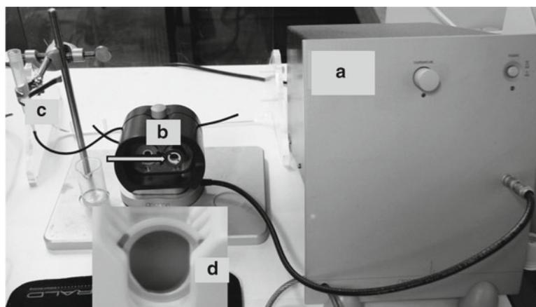
Fig. 1. The Q-sense (D-300) apparatus and its components. Shown are the electronic unit (a), measurement chamber (b), and the sample holder (c). The PS sensor crystal mounted on the 'O' ring of the measurement chamber is shown by an arrow near (b) and the smooth surface of the sensor crystal where AMs are adsorbed is shown in the inset (d).
