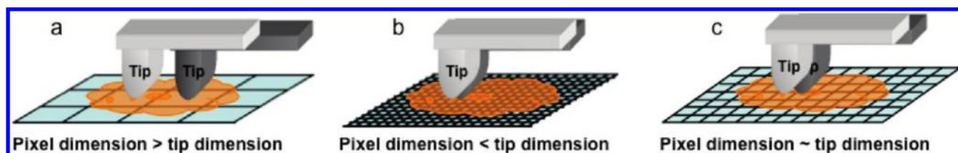
**Figure 7.** Schematic illustration of probe resolution in affinity mapping. An AFM probe addresses proteins on a cell membrane when the pixel dimension is greater than (a), less than (b), or approximately the same as (c) the tip dimension. The probe resolution is limited by the probe dimension.
