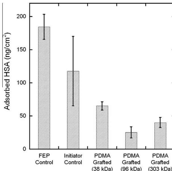
**Fig. 8.** Eu-tagged HSA adsorbed onto experimental FEP surfaces. Surfaces were incubated with 0.1 mg ml<sup>-1</sup> Eu-HSA in PBS for 18 h, then exhaustively washed and blown dry with nitrogen. Enhancement solution was incubated with the surfaces allowing for dissociation of the europium tag. Aliquots were quantified in a time-resolved fluorescence assay.
