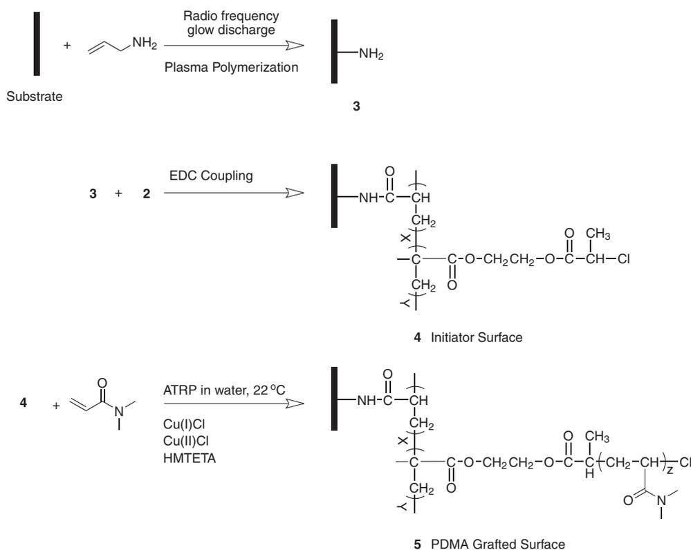
Fig. 2. Modification schematic for initiator functionalization and polymer grafting.
