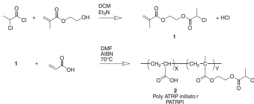
Fig. 1. Schematic illustration for the synthesis of PATRPI.
