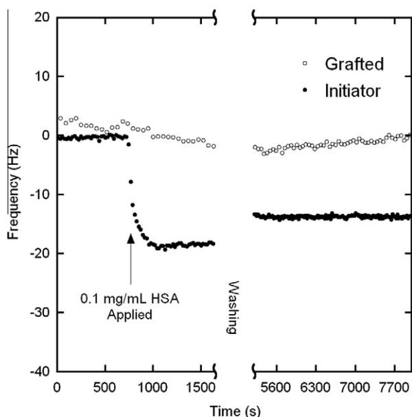
**Fig. 7.** QCM-D experiment demonstrating the effect of applying 0.1 mg ml<sup>-1</sup> HSA (indicated by the arrow) to substrates functionalized with either initiator or PDMA grafted polymer ([DMA] = 0.5 M). Washing involved at least 5 min applications of buffer, 1 M NaCl and water, followed by re-equilibration in buffer. Frequency shifts to lower values correlate with an increase in mass coupled to the surface.
