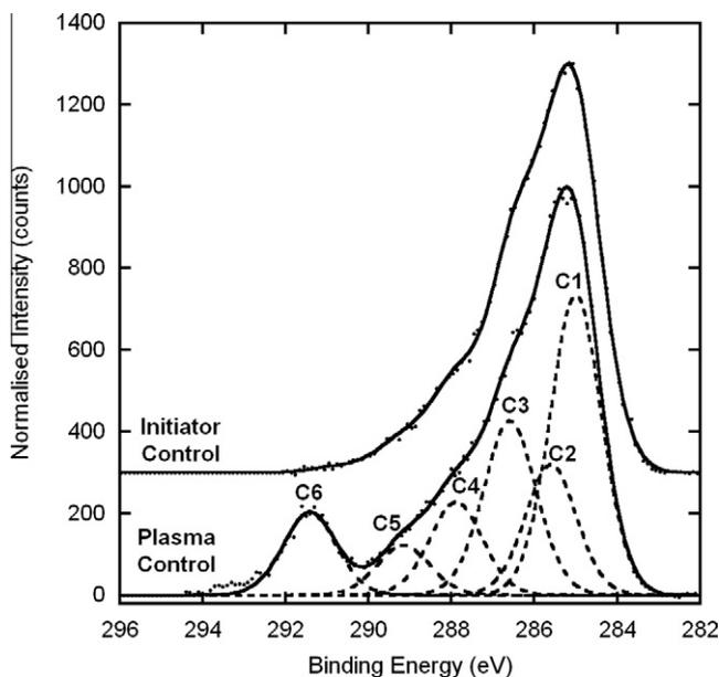
**Fig. 3.** High-resolution XPS scan of the C1s region of FEP substrates functionalized with allylamine plasma polymer (plasma control) or PATRPI copolymer (initiator control). Curve fits to the data comprising six components (dashed lines) are shown for the plasma control as an example.
