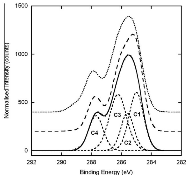
**Fig. 5.** High-resolution XPS scan of the C1s region of PDMA grafted from TCPS (top), FEP (middle) and Si wafer (bottom).
