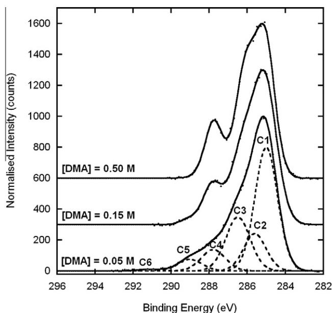
**Fig. 4.** High-resolution XPS scan of the C1s region of FEP substrates with different monomer concentrations. Curve fits to the data comprising six components (dashed lines) are shown for the [DMA] = 0.05 M graft layer as an example.
