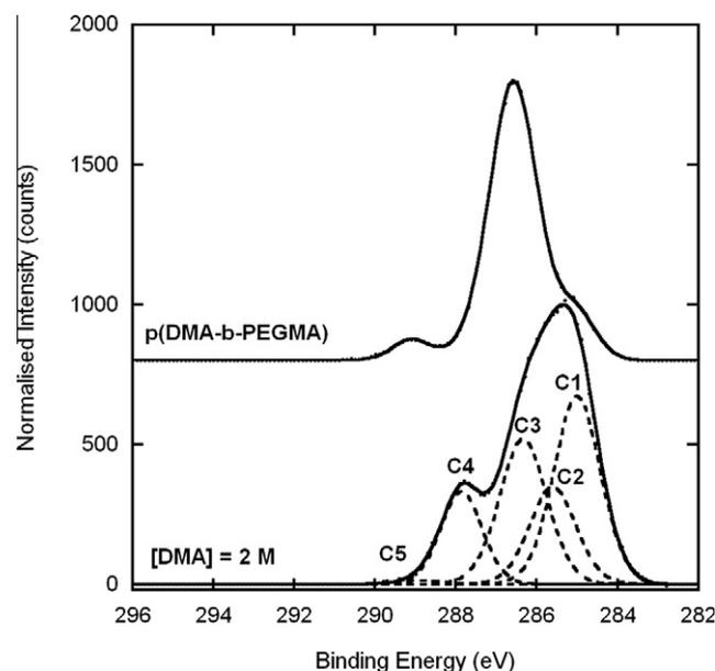
**Fig. 6.** High-resolution XPS scan of the C1s region of a silicon wafer grafted with [DMA] = 2 M (lower curve). When this surface was washed, dried and then introduced to a new solution containing fresh solvent, catalyst and [PEGMA475] = 1 M, a block copolymer was produced with a spectrum (upper curve) which was characteristic of PEGMA475 polymer. Curve fits to the data comprising six components (dashed lines) are shown for the [DMA] = 2 M grafted sample as an example.
