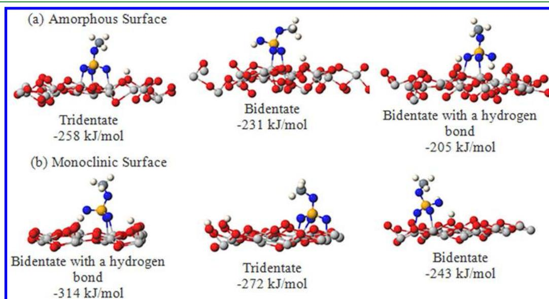
**Figure 6.** Illustration of DFT adsorption geometries for methyl phosphoric acid over the (a) amorphous and (b) monoclinic surfaces. Light gray spheres represent Hf atoms, red spheres represent O atoms of the surface, white spheres represent H atoms, dark gray spheres represent C atoms, orange atoms represent P atoms, and blue spheres represent O atoms of the phosphoric acid.
