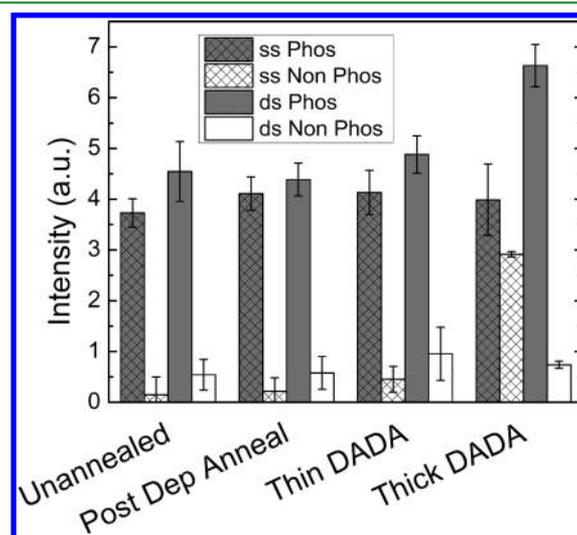
**Figure 3.** Relative fluorescence intensity of fluorescently labeled DNA spots on various ALD hafnium oxide surfaces. Dark bars indicate spots of phosphorylated DNA, and cross-hatching indicates single stranded DNA.
