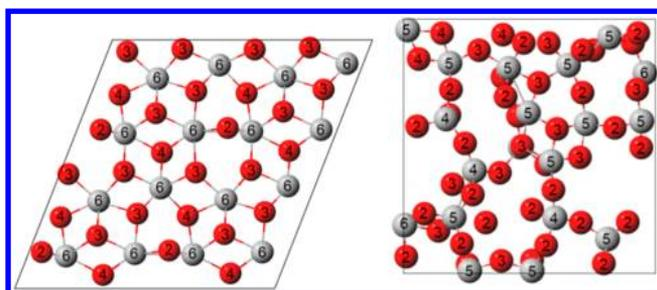
**Figure 1.** Top views of the monoclinic  $[111]$  (left) and amorphous  $[001]$  (right) surfaces of  $\text{HfO}_2$ . Numbers indicate the coordination number of the surface atoms. Gray spheres represent Hf atoms, and red spheres represent O atoms.
