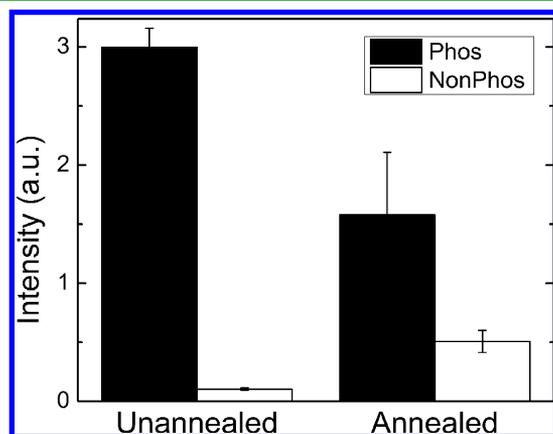
**Figure 2.** Dependence of DNA immobilization and hybridization on terminal phosphorylation state. Relative PicoGreen fluorescent intensity of phosphorylated (solid bars) and nonphosphorylated DNA spots after hybridization on annealed and unannealed ALD hafnium dioxide.
