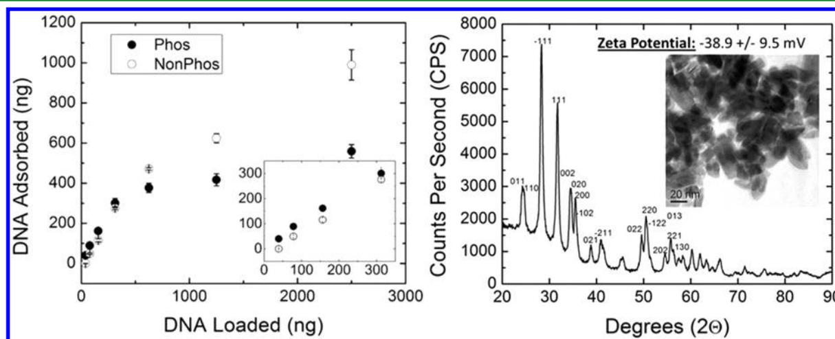
**Figure 8.** (left) Adsorption of phosphorylated and nonphosphorylated ssDNA on hafnium oxide nanoparticles. (right) Characterization of hafnium oxide nanoparticles including XRD peak identification of monoclinic peaks, TEM micrograph, and zeta potential of the surface of the particles.
