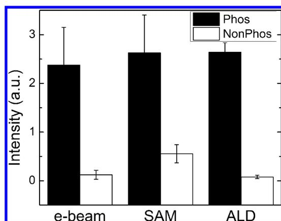
**Figure 7.** Relative fluorescence intensity of fluorescently labeled phosphorylated (solid bars) and nonphosphorylated DNA spots on hafnium-containing surfaces: e-beam evaporated hafnium oxide (e-beam), self-assembled monolayers of hafnium ion (SAM), and unannealed atomic layer deposition of hafnium oxide (ALD).
