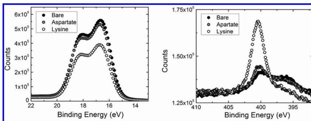
**Figure 4.** X-ray photoelectron spectroscopy scans of the Hf 4f (left) and N 1s (right) regions. Solid black markers represent the bare hafnium dioxide substrate, gray markers are the hafnium dioxide patterned with poly aspartate, and white markers are the hafnium dioxide patterned with poly lysine.
