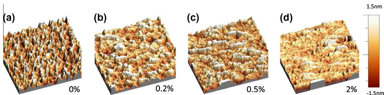
Fig. 3. AFM tapping analysis of  $\text{Si}_3\text{N}_4$  substrates immersed for 1 h into different concentrations of CTES.
