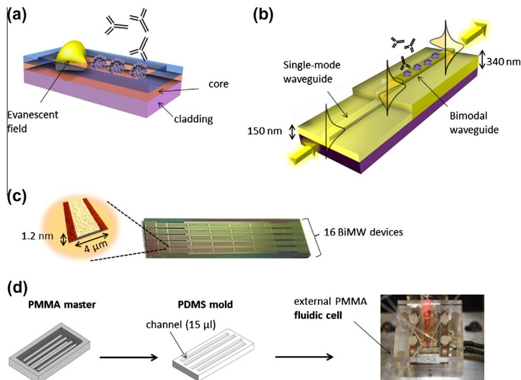
**Fig. 1.** (a) Scheme of the evanescent field detection principle in which the waveguide biosensors are based on, (b) interferometric operation of the BiMW device, (c) photograph of a chip consisting of 16 BiMW devices and AFM image of one rib waveguide, and (d) fabrication by soft-lithography of a PDMS mold and assembly of the fluidic cell using an external PMMA housing.
