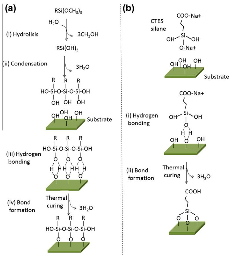
Fig. 2. Comparison between the silanization processes of surfaces using: (a) trialkoxyxilane, and (b) CTES silane.
