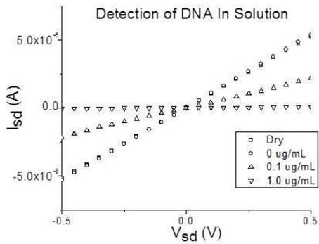
**Figure 2. Top:** Current-voltage (IV) curves showing an increase in source-drain resistance ( $R_{sd}$ ) as increasing concentrations of DNA cover the exposed gate dielectric. **Bottom:** IV curves of devices before and after printing with DNA in a biological buffer (left) and printing with buffer alone (right). Both were then rinsed with buffer and measured again.  $R_{sd}$  remains decreased on the DNA printed device, whereas the buffer control device does not show a significant response.
