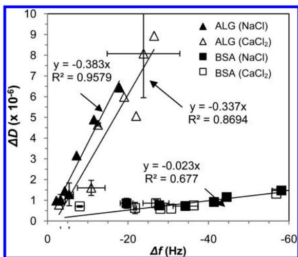
**Figure 3.** Measured dissipation change ( $\Delta D$ ) and frequency change ( $\Delta f$ ) at adsorption equilibrium.
