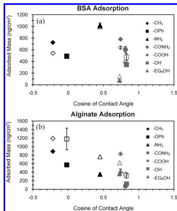
**Figure 1.** Calculated adsorbed mass of (a) BSA, and (b) sodium alginate on different SAMs at adsorption equilibrium. Adsorption occurred in 10 mM NaCl (solid symbols) and 7 mM NaCl/1 mM CaCl<sub>2</sub> (open symbols).
