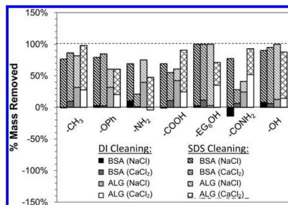
**Figure 4.** Stacked bar graph indicating % mass of adsorbed layer removed by DI (solid) and 2% SDS cleaning (pattern).
