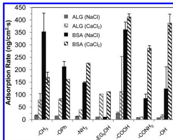
Figure 2. Initial adsorption rate of BSA and alginate.
