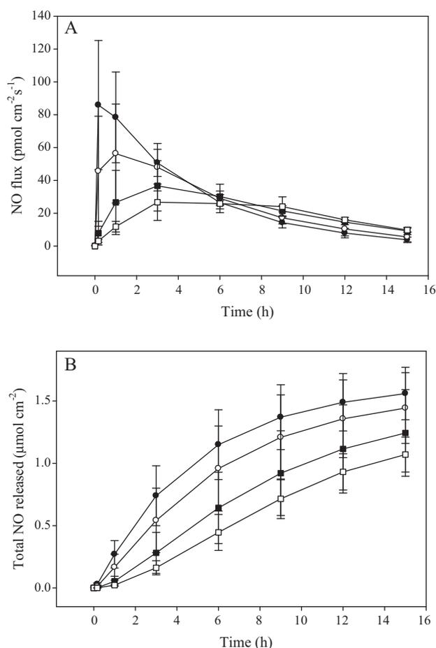
**Fig. 1.** (A) Nitric oxide flux and (B) NO totals from AEAP3/TMOS particle-doped ( $0.6 \text{ mg cm}^{-2}$ ) PU films (●) without and with additional Tecoflex SG-80A (TPU) layer at (○) 20, (■) 40, and (□)  $60 \text{ mg mL}^{-1}$  concentration.
