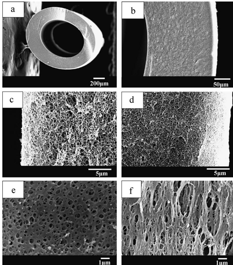
Fig. 2. SEM images of the hollow fiber membrane prepared by the TIPS method: (a) whole cross section; (b) enlarged cross section; (c) cross-section near the inner surface; (d) cross-section near the outer surface; (e) inner surface; (f) outer surface.
