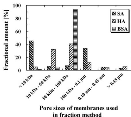
Fig. 4. Apparent molecular weight distributions for sodium alginate (SA), humic acid (HA) and BSA solutions.
