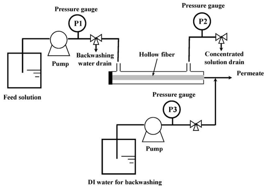
Fig. 1. Diagram of filtration-backwashing experiments using a single hollow fiber module.
