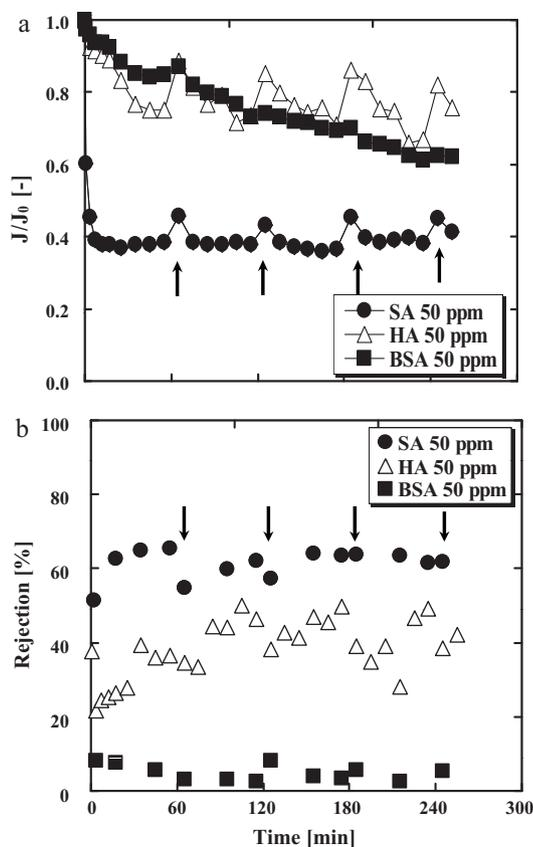
Fig. 3. Relative permeability (a) and rejection (b) as a function of filtration time for 50 mg/L sodium alginate (SA), humic acid (HA) and BSA solutions. Arrows in the figure show the backwashing process.
