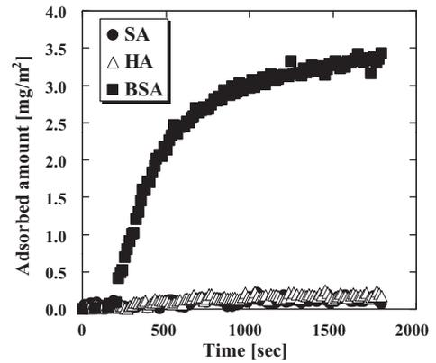
Fig. 6. Amounts of sodium alginate (SA), humic acid (HA) and BSA adsorbed on CAB spin-coated quartz crystal sensors as a function of time.
