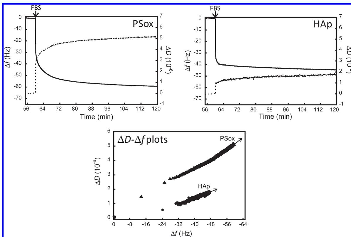
**Figure 2.**  $\Delta f$  and  $\Delta D$  curves and  $\Delta D-\Delta f$  plots of FBS preadsorption on PSox and HAp.  $\Delta f$  was transformed into the value for the fundamental frequency of 5 MHz by dividing by 3, which was the harmonic overtone number.
