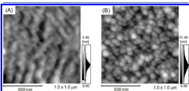
**Figure 1.** AFM topographic images of (A) PSox and (B) HAp over an area of  $1 \times 1 \mu\text{m}^2$ .
