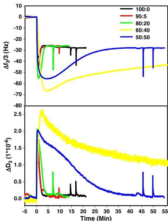
Fig. 2. QCM-D response during adsorption of DEPC:DMPG vesicles onto silica in "calcium-free" buffer.
