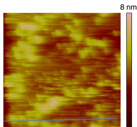
**Fig. 3.** AFM tapping-mode “snapshot” height image of 50:50 DEPC:DMPG vesicles adsorbed on a silica wafer and fusing to form a SPB in “calcium-free” buffer after rinsing. Exposure time was 15 min. SUV concentration was 0.125 mM. Image size was  $1.3 \mu\text{m}$ . Vesicles (circular objects) and bilayers (flat areas) were observed.
