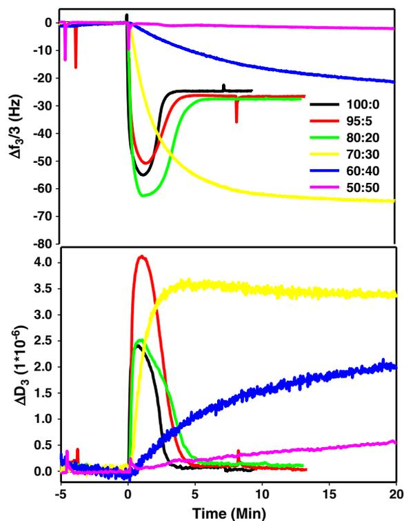
**Fig. 1.** Changes in QCM-D response for the 3rd overtone frequency, 15 MHz, (top) and its corresponding dissipation (bottom) for the adsorption of DEPC:DMPG SUVs at 100:0 (black line), 95:5 (red line), 80:20 (green line), 70:30 (yellow dotted line), 60:40 (blue line), and 50:50 (pink line) molar ratios onto silica in the presence of 2 mM  $\text{CaCl}_2$ , 10 mM TES, and 150 mM NaCl at pH 7.4.
