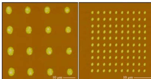
Figure 1. AFM images of a UV curable adhesive (Norland optical adhesive #81) arrayed on a silicon surface. The left hand panel shows an array of spots approximately 6 μm in diameter with a pitch of 15 μm. The right hand panel shows an array of spots approximately 1 μm in diameter with a pitch of 3 μm.
