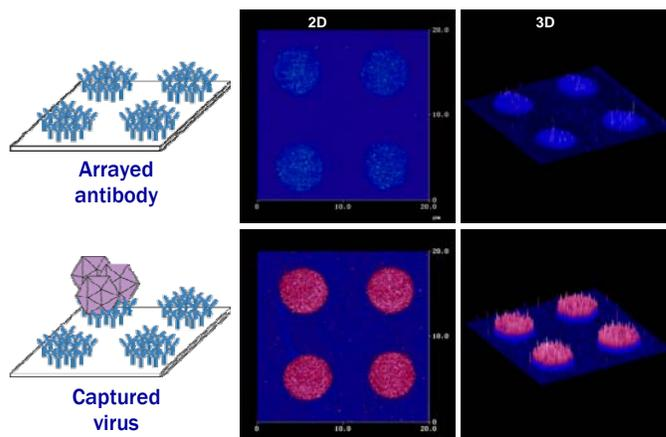
Figure 1. Group B Coxsackievirus capture and detection on antibody spots with AFM. The left panel shows a graphic depiction of negative (top) and positive (bottom) whole virus capture process with 2D and 3D AFM views for each on the right.
