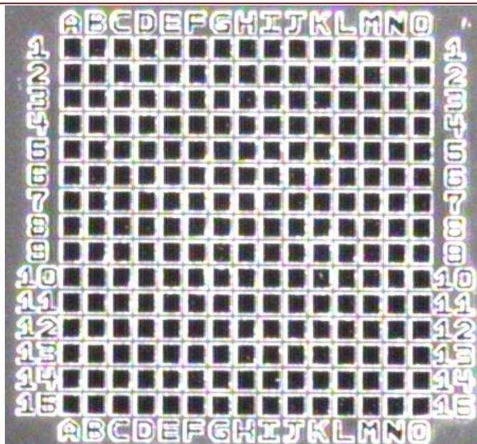
Figure 1: Optical image of the indexed grid portion of a 4mm Sindex™ chip. Individual silicon pads measure 100  $\mu\text{m}$  x 100  $\mu\text{m}$  and may be coated with metals or functionalized with additional surface chemistries.
