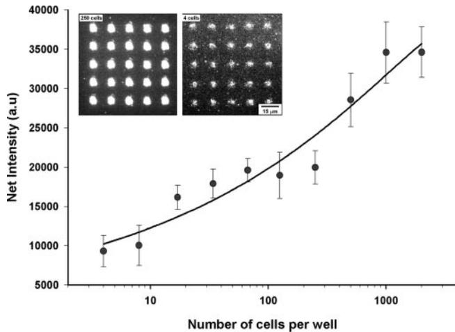
FIG. 4. **PSA detection from a model cell culture system.** 2-fold serial dilutions of LNCaP cells were grown in 1,536-well plates, and the supernatant was collected after 24 h. The supernatant was assayed for PSA, and the relationship between net fluorescence signal intensity and number of cells was plotted. Each point is the average of at least three trials. The *inset* shows the raw fluorescence data from 250 (*left*) and four (*right*) cells.
