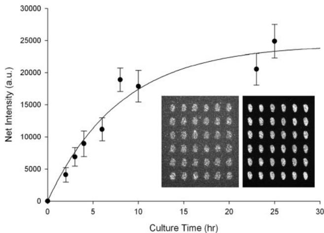
FIG. 5. **PSA detection from LNCaP cell as a function of time.** LNCaP cells were cultured in 1,536-well plates with 100 cells/well for the indicated times. The supernatant was collected and assayed for PSA. The net fluorescence signal intensity was plotted as a function of time. The *inset* shows the raw fluorescence intensity at 2 h (*left*) and 23 h (*right*).
